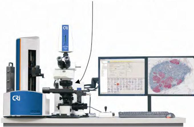
High-res spectral imaging & automated scanning of the whole tissue section
