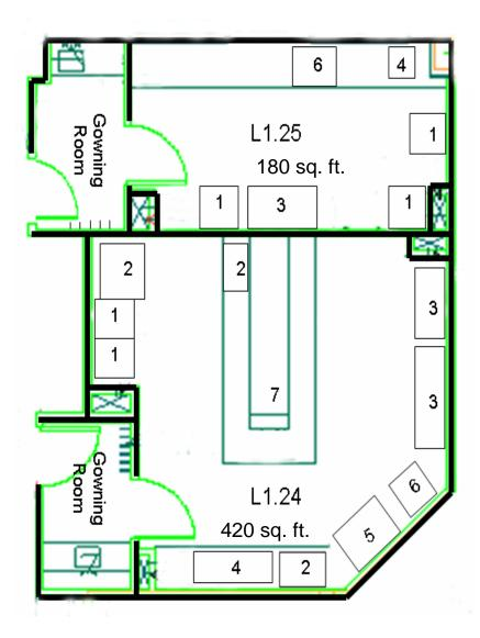
The floor plans and equipment in two of the three cleanrooms
